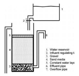
Over time, however, the sand media in the filter will become fouled. As a result of this fouling, it becomes difficult for wastewater to percolate through the filter media. In such an instance, wastewater can suddenly pool on the filter and overflow the system.
