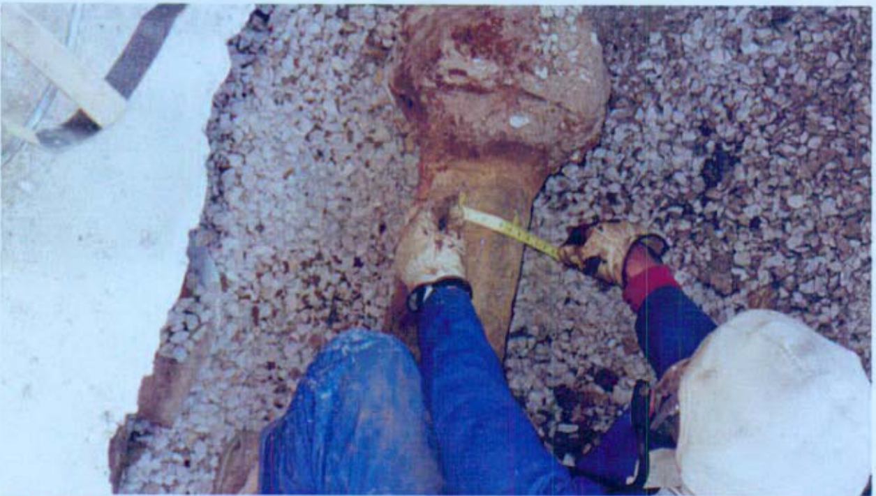
Photograph 4 – View of circumferential crack in 6-inch cast iron main. The crack extended from the 1 o'clock position to the 11 o'clock position. The worker's left thumb marks the 11 o'clock position.
