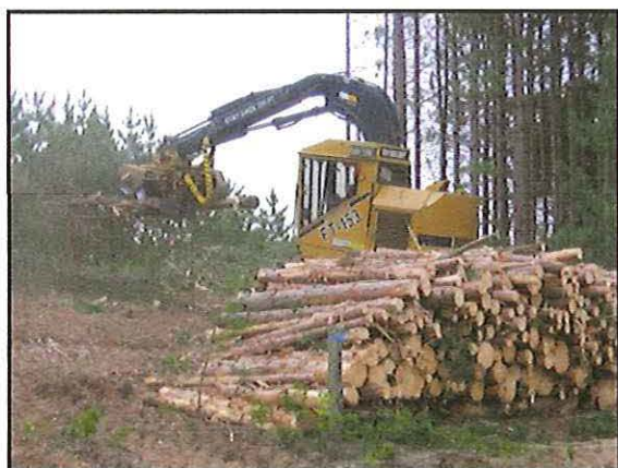
Figure 9 Whole Tree Processor Clearing
