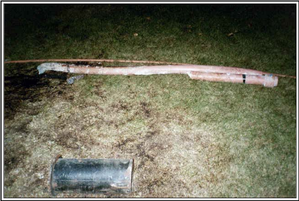
Photograph 5: View of the burned segments (in the background) of 3-inch diameter PE natural gas piping that were removed from the excavation on the evening of 9/25/02.
