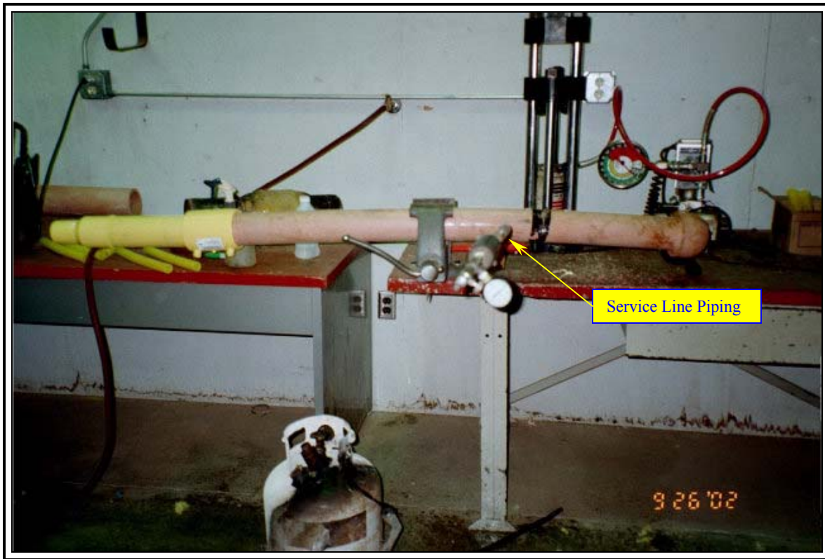
Photograph 9: Pressure test of the intact portion of 3-inch diameter PE natural gas main and tapping tee with service line piping (small segment) that served 1910 E. Burntwood Street. This natural gas piping was removed from the excavation in front of 1904 E. Burntwood Street on 9/26/02. A new section of yellow PE piping was added (upper left side of photograph) to facilitate the pressure test.
