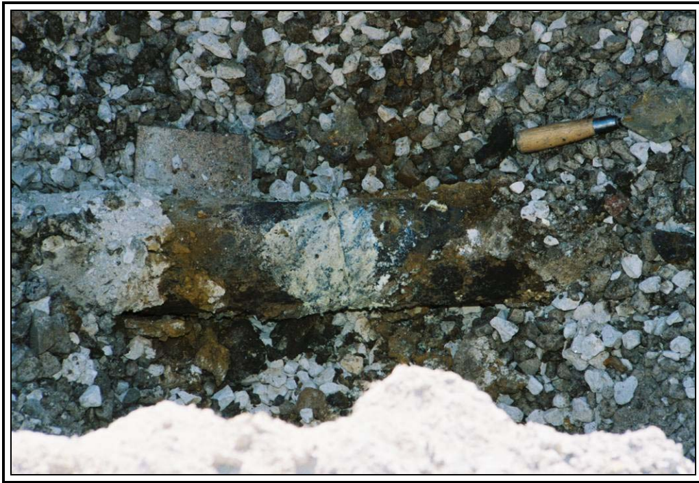
Photograph 3 View looking inside of the excavation along Steins Street after the concrete patch for the street was removed on December 30, 2008. Observe the fracture area around the circumference of the 4-inch natural gas CI main.
