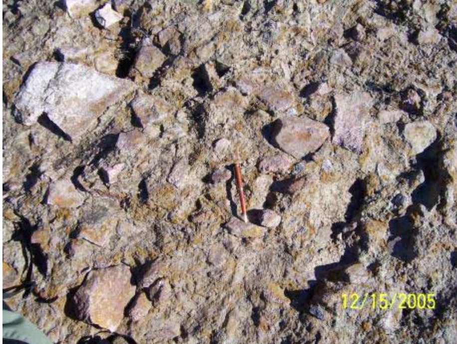
Figure 2.6 - Foundation area composed of weathered rhyolite with some clay, located in breach area.
