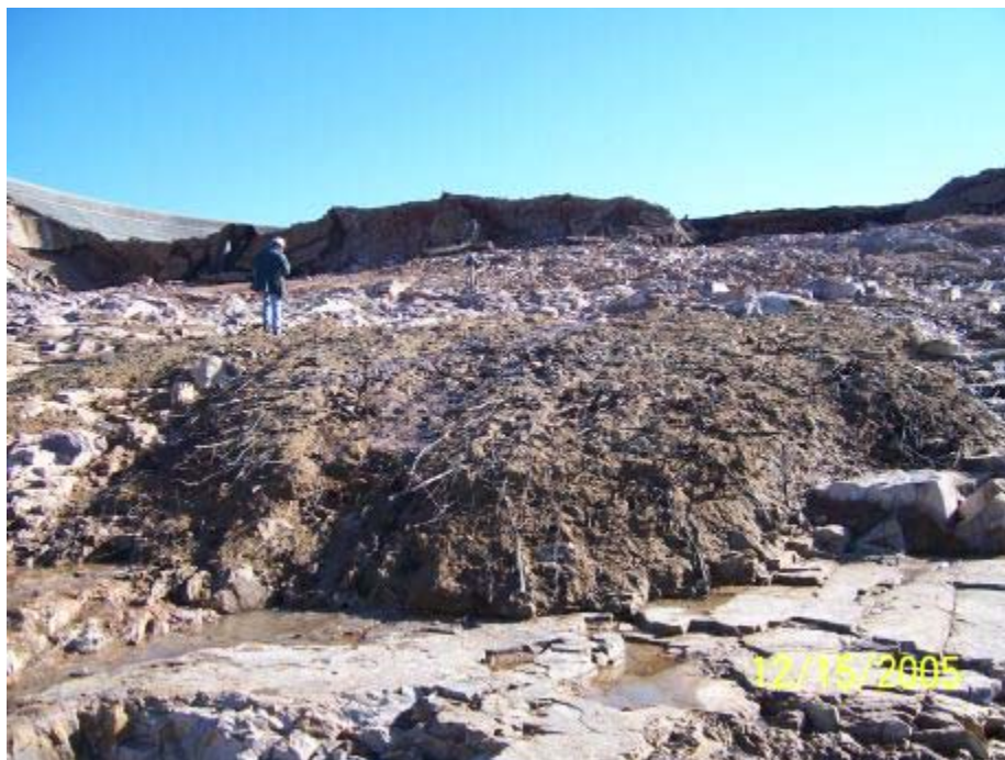
Figure 9.3 - Residual topsoil on top of fresh rhyolite.
