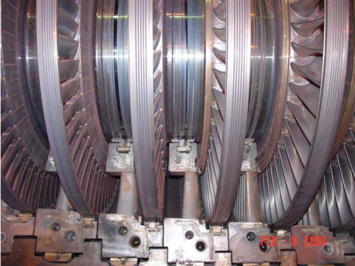
HP Interstage Diaphragm Packing Damage
