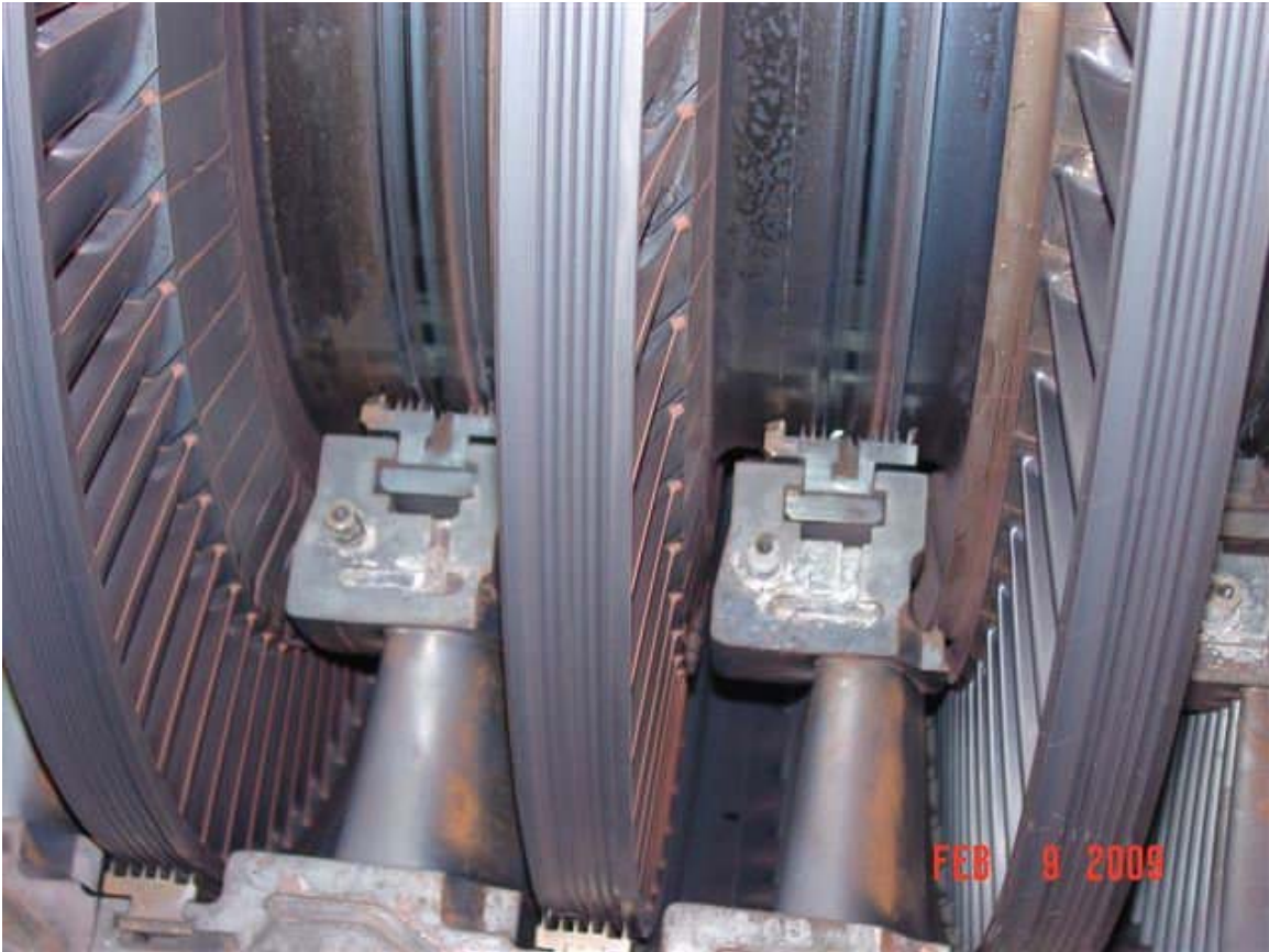
HP Interstage Diaphragm Packing Damage
