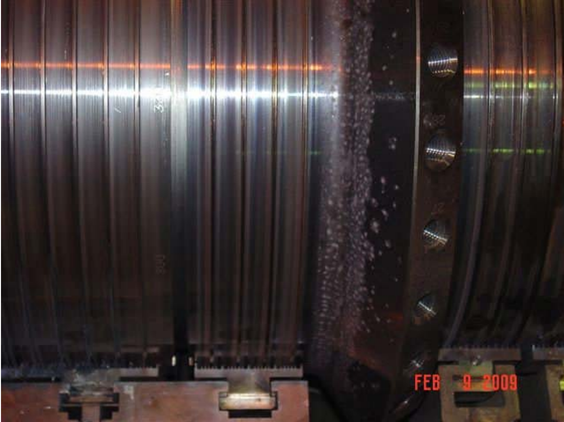
HP N1 Packing Casing Wear
