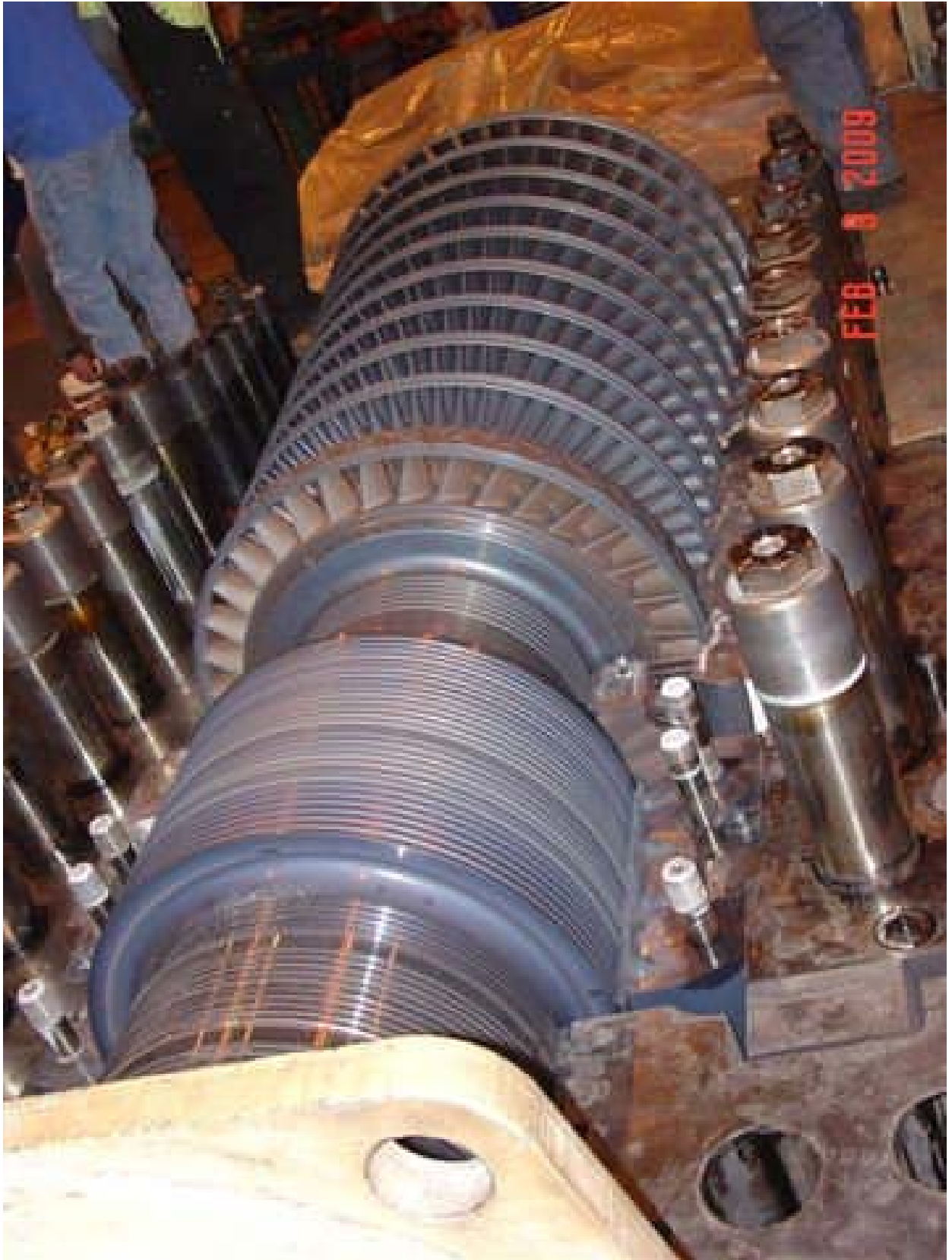
HP Rotor with UH Diaphragms Removed
