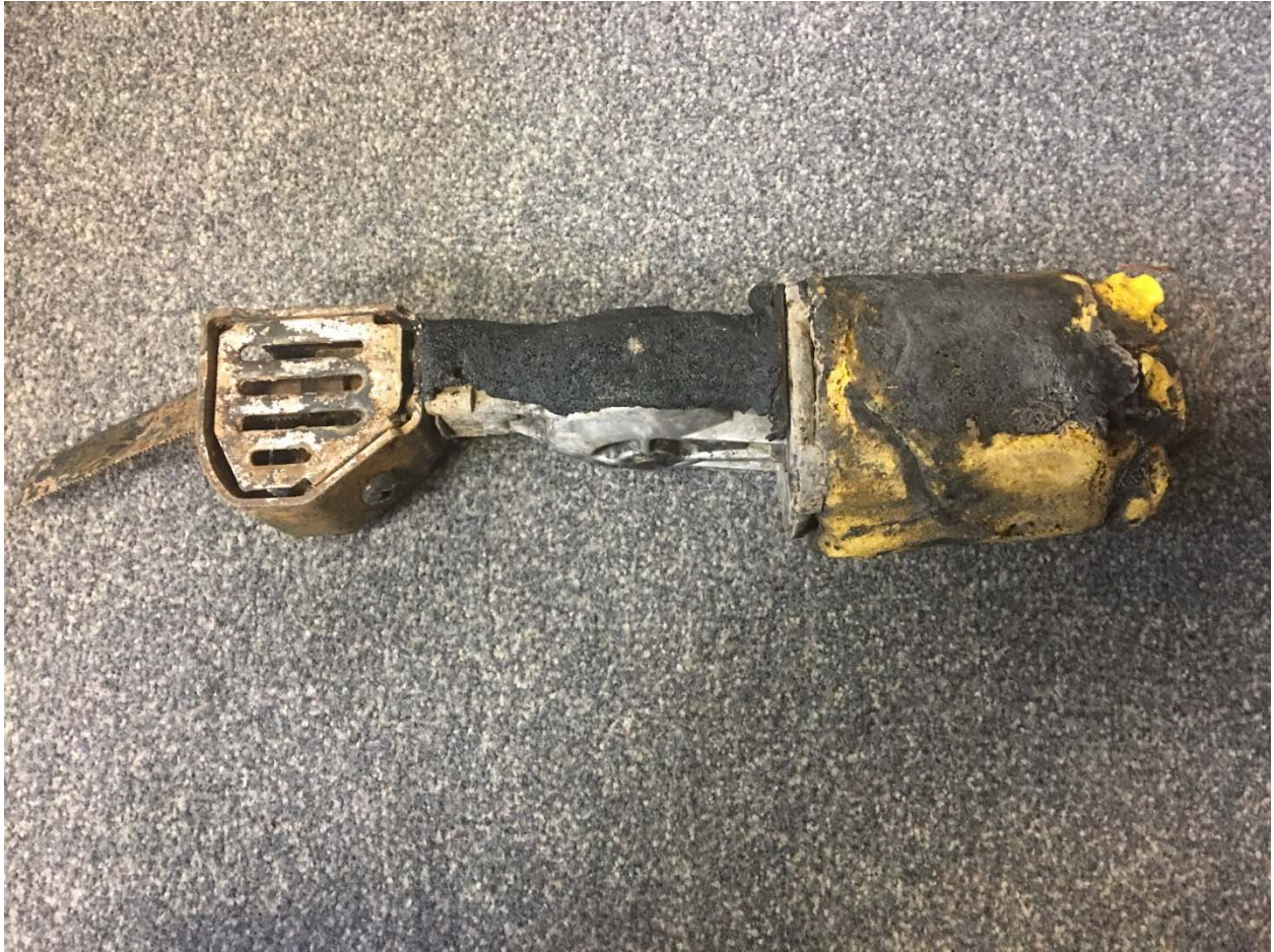
Photograph 2: Photograph of electric reciprocating saw following the incident (Source: Spire, confirmed in Spire response to Staff Data Request 0061).
