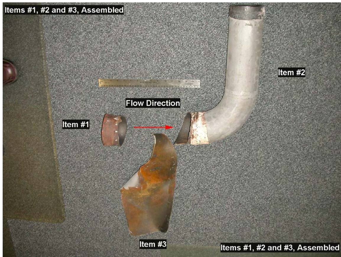
Figure 5.2 – Failed 4 inch SH Attemperator Spray A-Line
