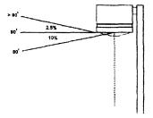
**88-430-05-B.** Light fixtures mounted under gas station canopies must be completely recessed into the canopy with flat lenses that are translucent and completely flush with the bottom surface (ceiling) of the canopy.
