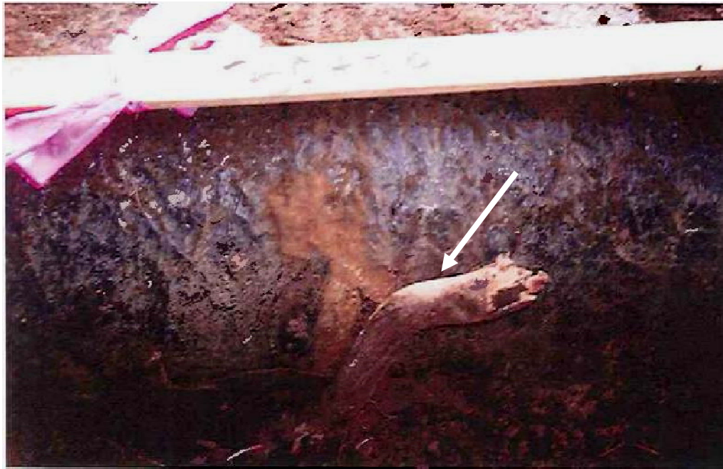
Example 1: Coating Damaged by Tree Root Intrusion (Arrow), Found in Excavation for Coating Defect No. 59, Active corrosion was observed under the coating. [45 dB \mu V (Minor, ACVG Score = 4); CIS “Off” = -0.867 (CIS Score = 5), Total ECDA Score = 11].
