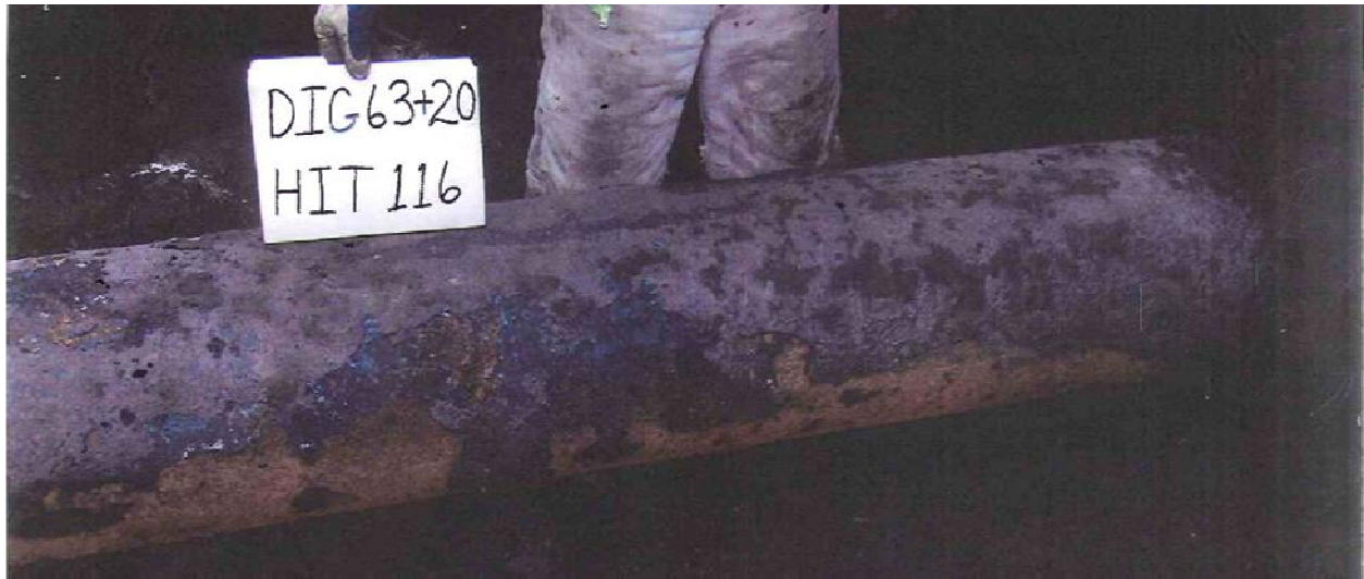
Example 3: Coating Not Properly Applied, Found in Excavation for Coating Defect No. 116, No Coating Applied to Sides, [47 dB \mu V (Minor, ACVG Score = 4); CIS “Off” = -0.855, “On” = -0.907 (CIS Score = 5), Total ECDA Score = 11].
