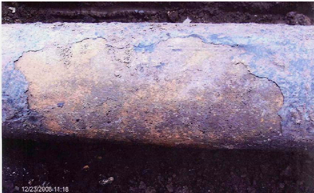
Example 2: Coating Disbonded, Found in Excavation for Coating Defect No. 137, [64 dB \mu V (Moderate, ACVG Score = 6); CIS “Off” = -0.821, “On” = -0.842 (CIS Score = 10), Total ECDA Score = 18].
