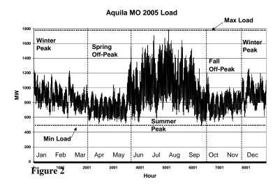
Plants built to operate **most of the time** are called **Base Load** plants. Plants built to operate **some of the time** are called **Intermediate** plants, while those that operate only a smaller **part of the time** are called **peaking** plants.
