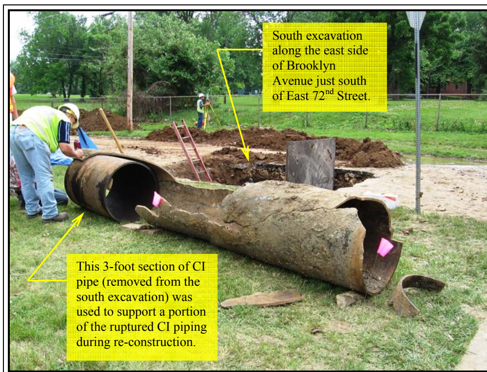
Photograph 4 Looking southwest at the various pieces of 24-inch diameter CI main that the Staff and MGE personnel were assembling. After assembling the ruptured sections of CI pipe, the measured length along the pipe's longitudinal axis from the north end to the south end was approximately 13 feet and 3 inches.
