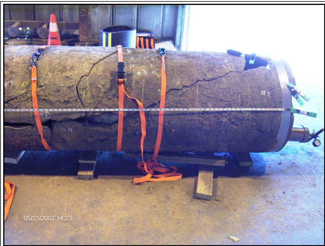
Photograph 1 View of a portion of the 24-inch diameter CI pipe fragments that were pieced together by MGE at their training facility. The duct tape wrapping near the right side is approximately where the mechanical coupling would have been located at the north end of the north excavation (Photograph provided by MGE).
