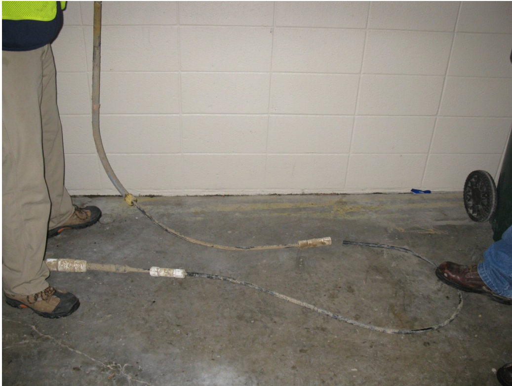
Photograph 3: Removed section of service line from 3404 Georgia Street following incident (Source: Staff Photograph taken November 28, 2015).
