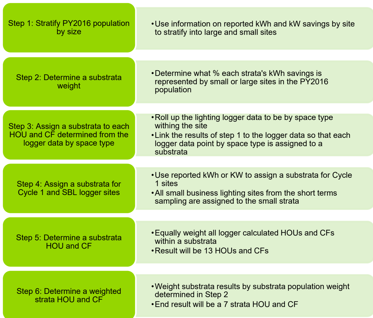
Figure E-1 Methodology for Determining Strata HOU and CF from Logger Data
