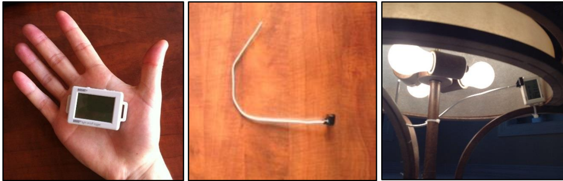
Figure 1. Left to Right: Light Meter; Fiber Optic Eye; Installed Meter and Fiber Optic Eye
