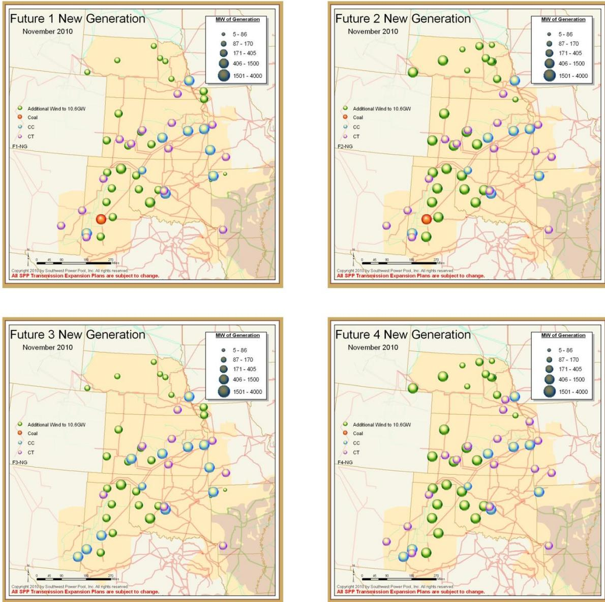
Figure A5.2: Additional Capacity Sites by Technology Type for each Future
