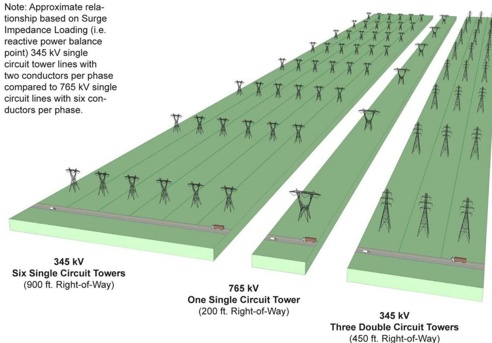
Figure 3.3: Relative right-of-way for equivalent loadability, courtesy AEP
