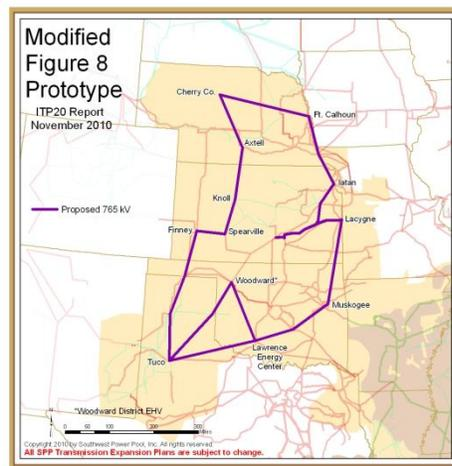
Figure 5.2: Modified Figure 8 Prototype
