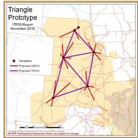
Figure 5.3: Triangle Prototype
