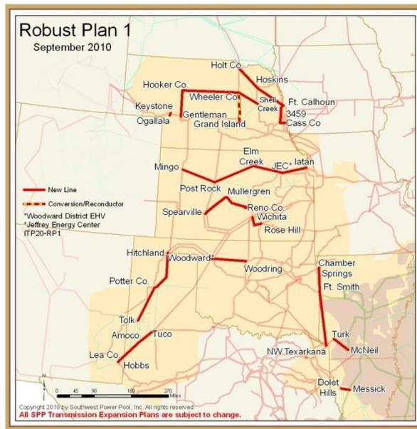
This plan enables SPP to respond to potential state and federal policy initiatives such as an RES or carbon mandate. Robust Plan 1 provides transmission upgrades in eight states in the SPP footprint. In addition to the previously described quantitative and qualitative value, the plan also addresses the SPPT's goals for transmission development for the ITP:
