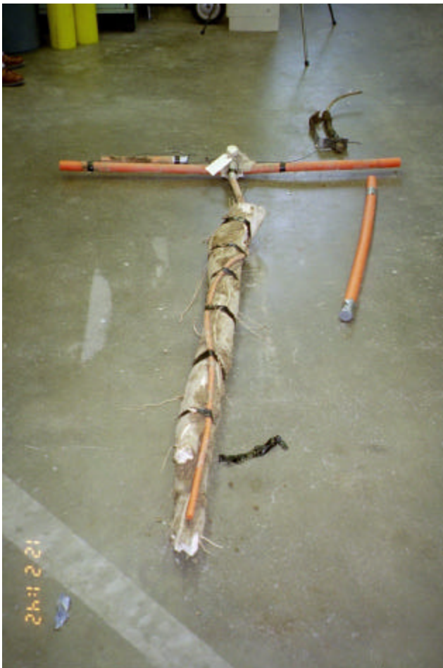
Photograph 13 Distribution main, service tee, service line and tracer wire serving #6 Hagers Mill Court.
