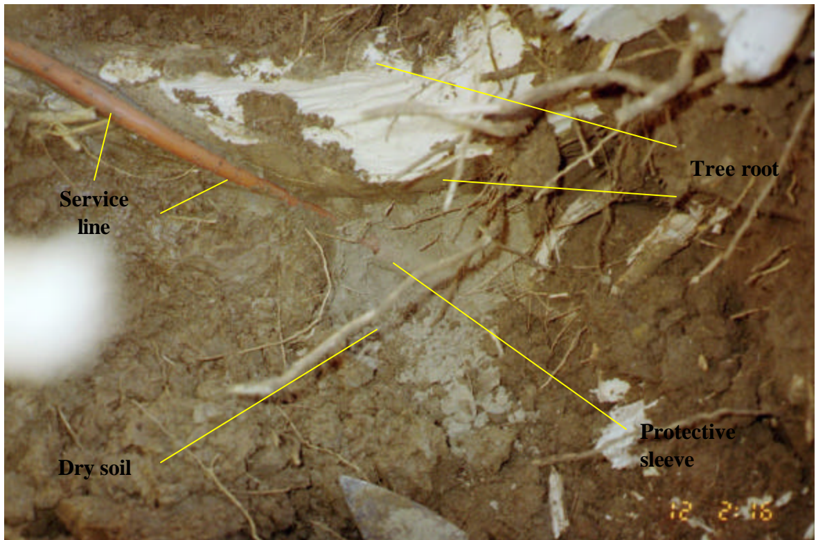
Photograph 10 Dry soil located under the tree root ball. The natural gas service line and protective sleeve can be seen in the soil.
