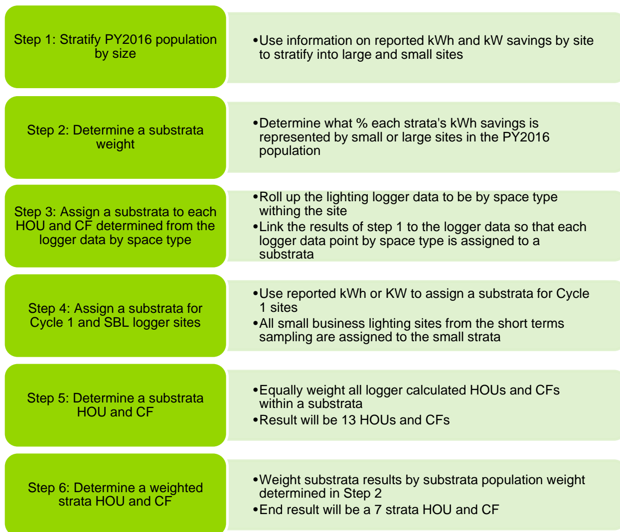
Figure E-1. Methodology for Determining HOU and CF from Logger Data
