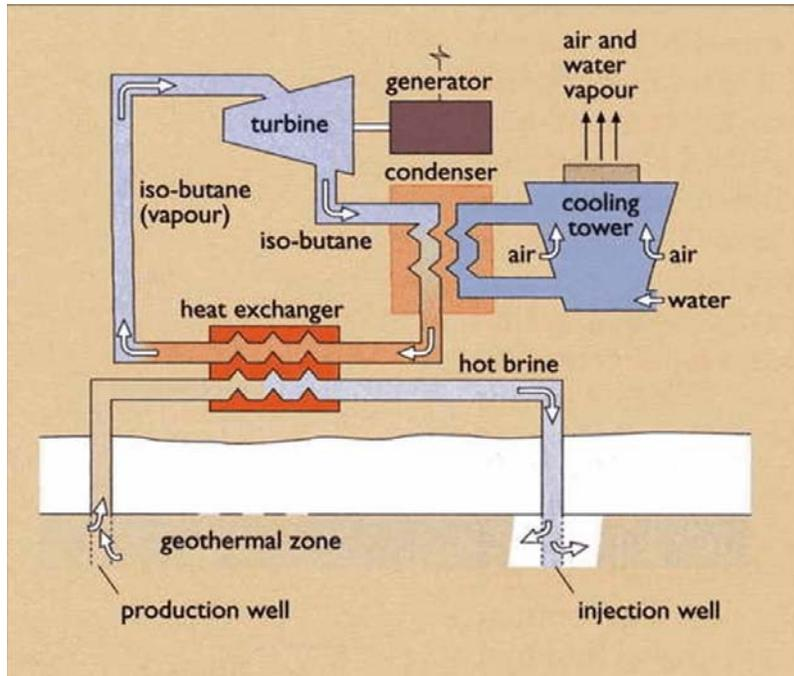
**Figure 24. Representative Geothermal Plant: Raft River Plant (Idaho)**
