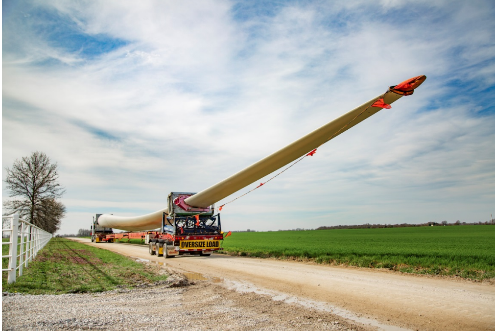
Picture 3. V 120 Turbine blade delivery.
