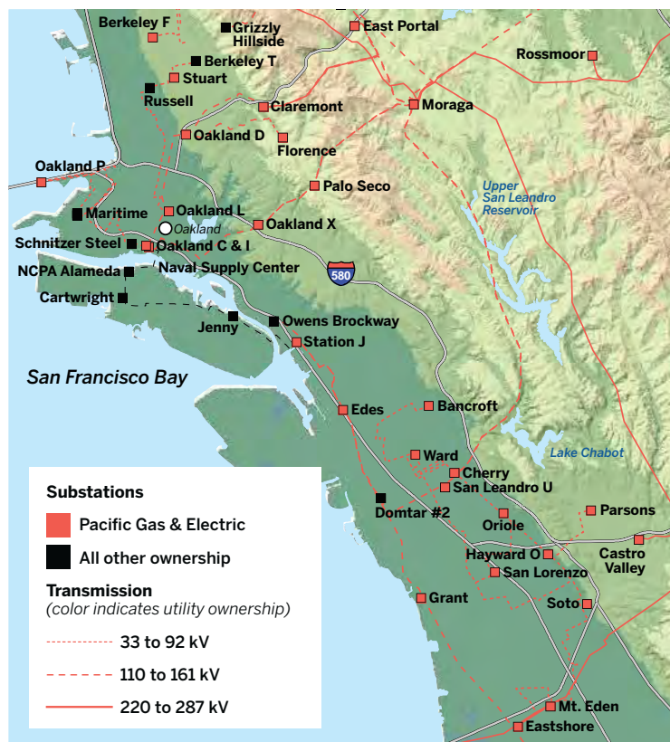
Figure 36. Transmission east of San Francisco Bay
