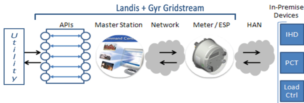
Figure 5: Communication Flow from Utility, through Gridstream, to the HAN via the Meter Gateway
