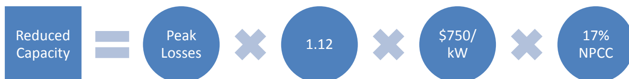
Figure 16.6: Calculating Reduced Capacity Cost Due to Losses
