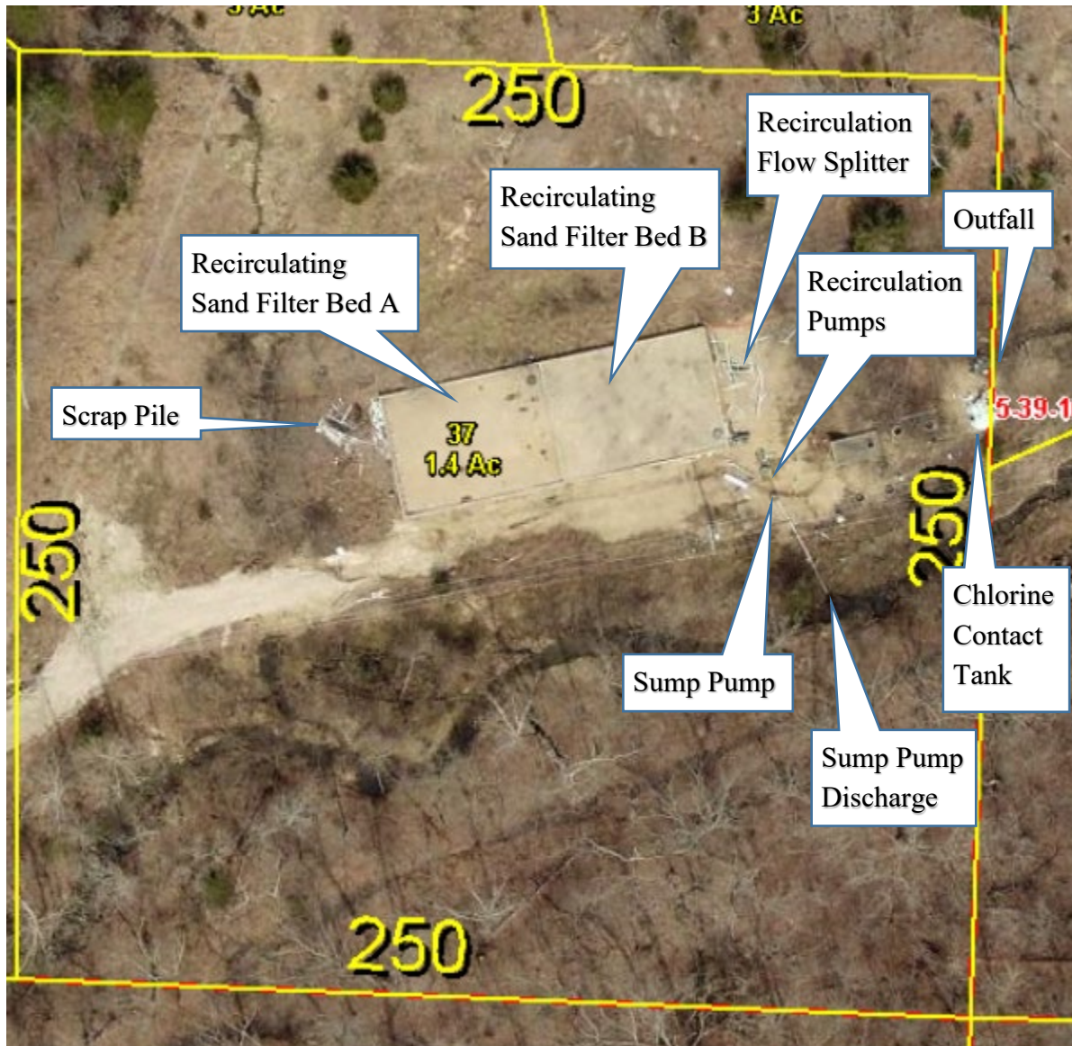
Figure 2: Aerial map of Osage Water Company KK WWTP courtesy of Camden County GIS System.
