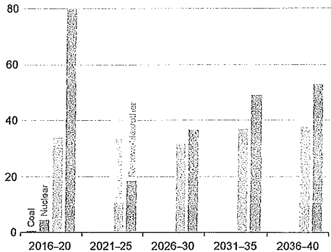
Figure MT-31. Cumulative additions to electricity generation capacity by fuel in the No CPP case by period (gigawatts)
