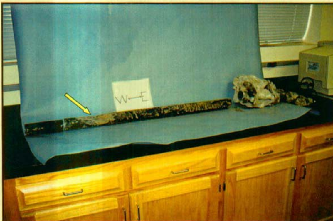
Photograph 6: View of the section of 2-inch OD coated-steel natural gas service line that was removed from the incident site. The arrow points to the area of damage. The east section of pipe, shown on the right of the photograph, still has some of the concrete encasement attached. This layer of concrete encased the service tee at the main to past the area where the service line was damaged.
