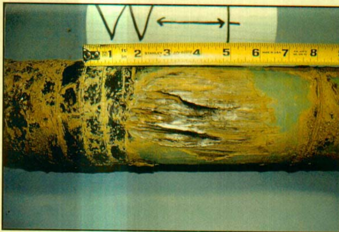
Photograph 4: Close-up view of the damage to the 3-inch OD coated-steel natural gas service line for 1204 Walnut.
