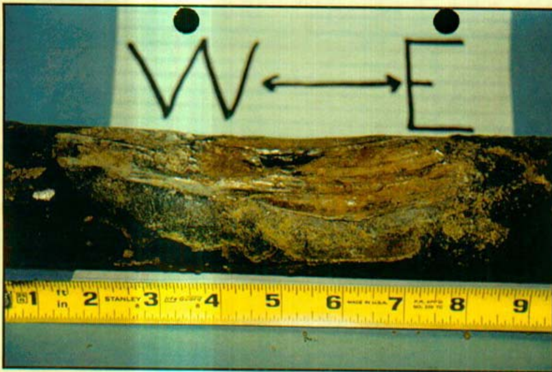
Photograph 7: Close-up view of the 2-inch OD coated-steel natural gas service line showing the damage and the approximate 1-inch by 1/2-inch hole. Natural gas escaped from this service line at a pressure of 30 inches water column.
