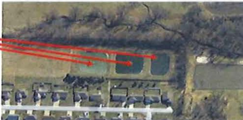
Original Three Cell Aerated Lagoon
