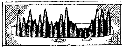
Figure 46 - Incorrect Burner Flame Pattern
