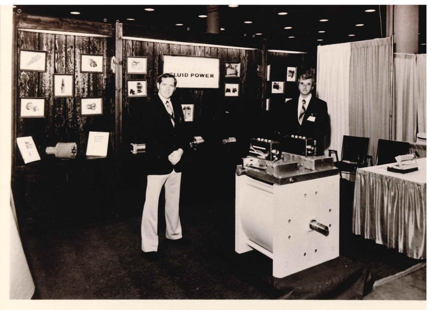
Hydraulic and Pneumatic show with 28" Bore cylinder which has complete manifold air circuitry for fail-safe main steam isolation valve operation. Shows redundant trains A&B, cylinder and air valve panel designed to withstand 110 PSI ambient pressure. Made for TVA Nuclear Power Stations Made 48 pieces
