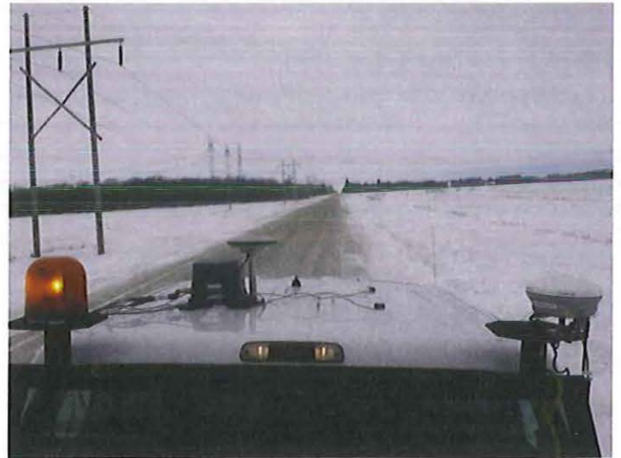
Figure 3 - Mobile GNSS, inertial, and RF equipment elements mounted on roof of test vehicle. Trimble R8 rover unit at bottom right, high sensitivity GPS antennas on roof at right, NovAtel 702 GG dome antenna center left directly adjacent to LCI IMU (gray box) at center left.
