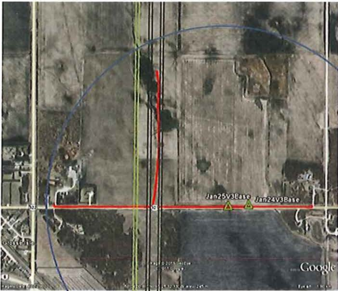
Figure 2 - Map of test location showing location of the NovAtel V3 base stations for each day (green triangles), range of Trimble R8 450 MHz data link (blue circle), and position of HVDC bipoles 1 and 2 (black lines), position of AC Line (green lines) and trajectory throughout the day of the test vehicle (red). Base map from Google (2011).
