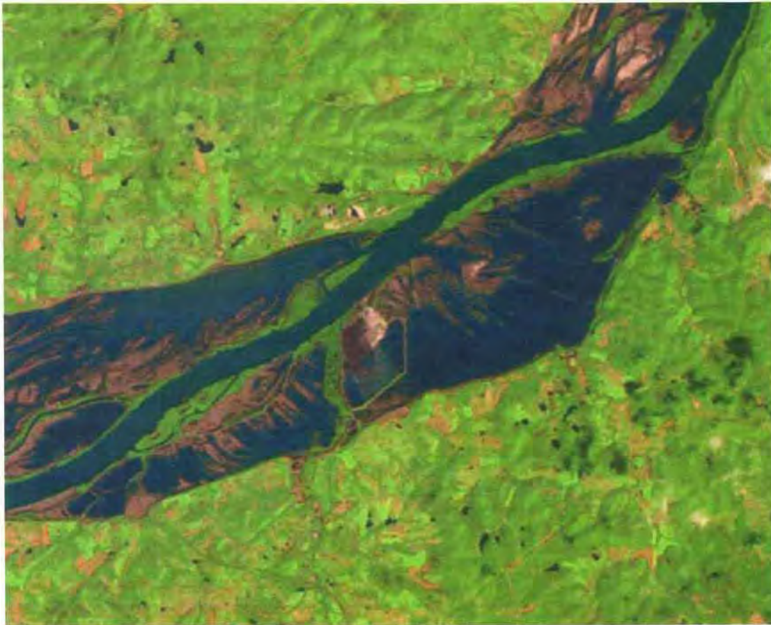
Figure 1. Detail of Labadie Bottoms on August 19, 1993, about 3 weeks after the flood peak of July 31 on the lower Missouri River. The river had overtopped the crest of the agricultural levee by more than 3 feet, inundating the bottoms. Although the river had fallen by more than 12 feet by the date of this satellite photo, the river was still higher than most of the bottomland, mostly situated at elevations between 465 and 471 feet MSL. The diamond-shaped area near the image center includes additional levees and encompasses the power plant, which has a high floor elevation of 491 ft. This figure shows an area of approximately 6 miles by 8 miles, detailed from Landsat 5/TM Image No. 114016 (NASA, 2010).
