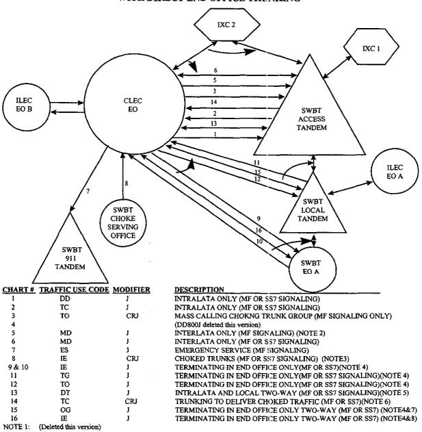
NOTE 2: Required at the Dallas 4 ESS switch only for 10xxx number cut through and Feature Group B over D
