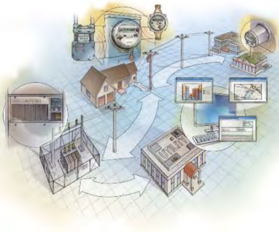
Figure 1-7: AMI RF Mesh FAN
