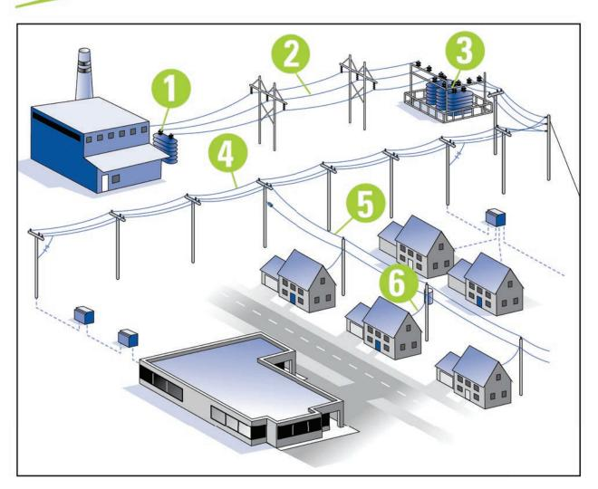
CP&L produces electric energy at our power plants using a diverse mix of fuels and technologies. The voltage produced is stepped up and the electricity is "pushed" into the grid or electric system using on-site substations.
