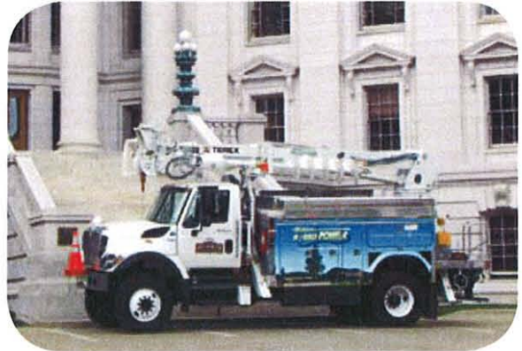
Plymouth Utilities' plug-in hybrid electric utility line truck.
