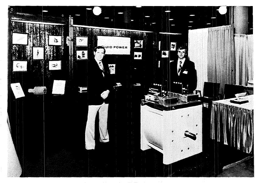
Systaulic and Pneumatic show with 28" Bore Cylinder which bas complete manifold air circuitry for fail-safe main steam isolation valve operation. Shows redundant trains A&B, cylinder and air valve panel designed to withstand 110 PSI achient pressure. Made for TVA Nuclear Power Stations Made 48 pieces
