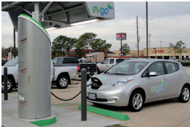
FIGURE 2-9 DC fast charging a Nissan Leaf. DC fast charging is able to charge a Nissan Leaf battery to 80 percent capacity in 30 min. The charge would typically allow a 2014 Nissan Leaf to travel about 67 miles. SOURCE: Copyright © 2010 by the eVgo Network, licensed under Creative Commons 2.0 (CC-BY-2.0).
