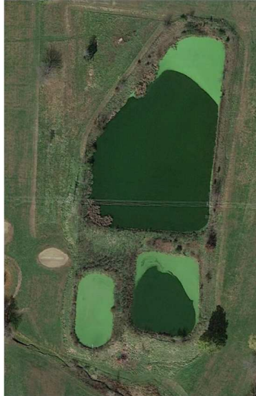
5 6 Aerial photo of lagoon system with visible overgrowth
