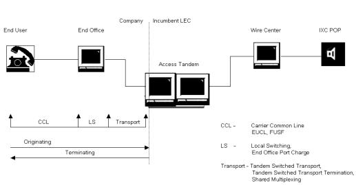
Figure 1 - Switched Access Rate Elements
