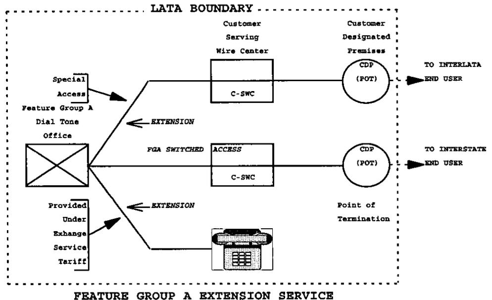
In the above example, two CDPs are utilized to better illustrate the concept. From a practical standpoint, both the Switched Access and Special Access Services could be routed via the same CDP.
