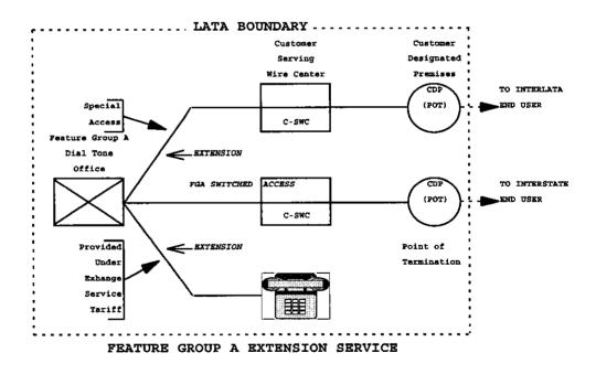
In the above example, two CDPs are utilized to better illusing the concept. From a practical standpoint, both the Switched Access and 7 Special Access Services could be routed via the same CDP.
