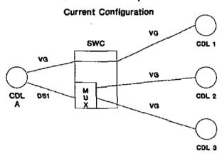
The customer requests that the voiceband circuit (VG) between CDL A and CDL 1 be "rolled over" to the DS1 serving CDL A. No NRCs apply for this request.
