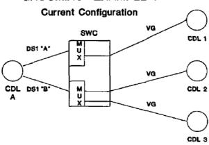
The customer requests that the voiceband (VG) circuit serving CDL 1 be moved from the DS1 "A" circuit to the DS1 "B" circuit. No NRCs apply for this request.
