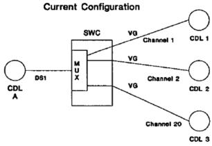
The customer requests that the voiceband circuit serving CDL 3 be moved from channel 20 in the DS1 serving CDL A to Channel 3 in the same DS1. No NRCs apply for this request.
