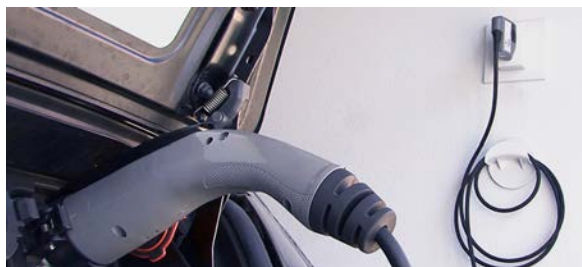
Photo 3. This EVSE cordset can be stored in a vehicle and plugged into an available electrical outlet. It can be used for Level 1 or Level 2 charging. Photo from AeroVironment.
