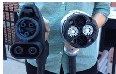
Photo 23. SAE J1772 CCS connector (left) and CHAdEMO connector (right). Photo from Margaret Smith.
