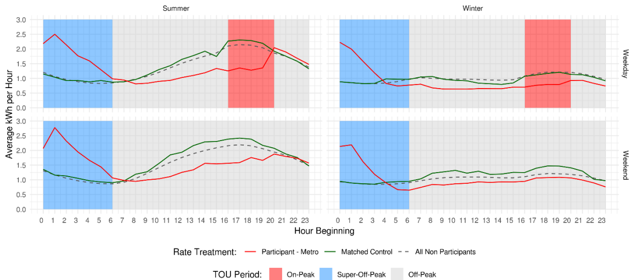
Figure 37. Electric Vehicle Post Period Load Shapes – Missouri Metro
