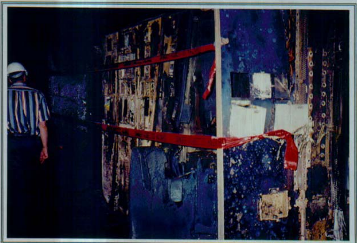
Equipment damaged by electrical ground fault
