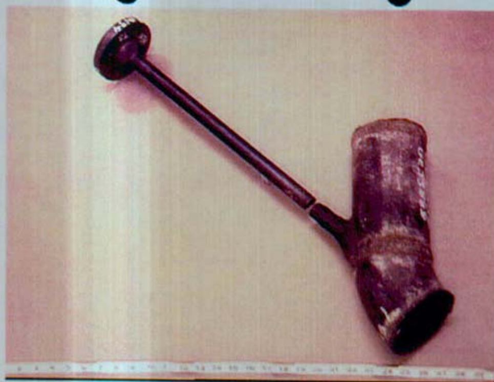
Figure 3 - This photograph shows the \frac{3}{4} " line that failed and the 4" main supply line. The bolted flange at the top of the photograph connects to the power oil relay.
