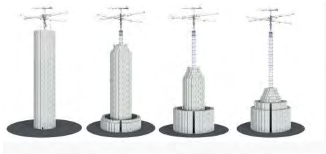
Figure 6.11 Concrete Block Storage System – Fully Charged to Fully Discharged 15
