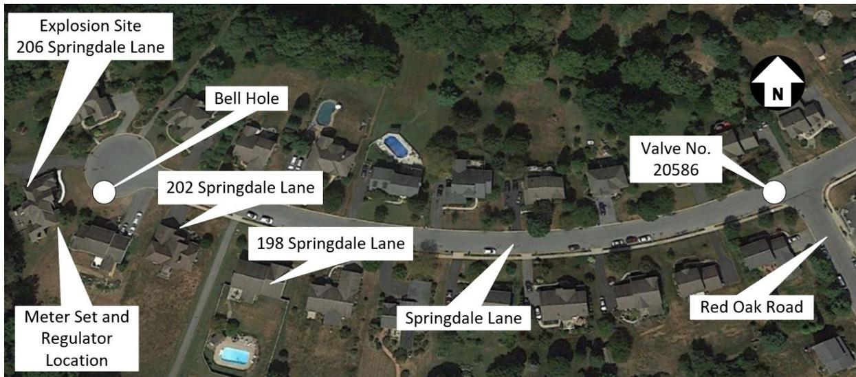
**Figure 2.** Location of gas shut-off valve in relation to accident site.
